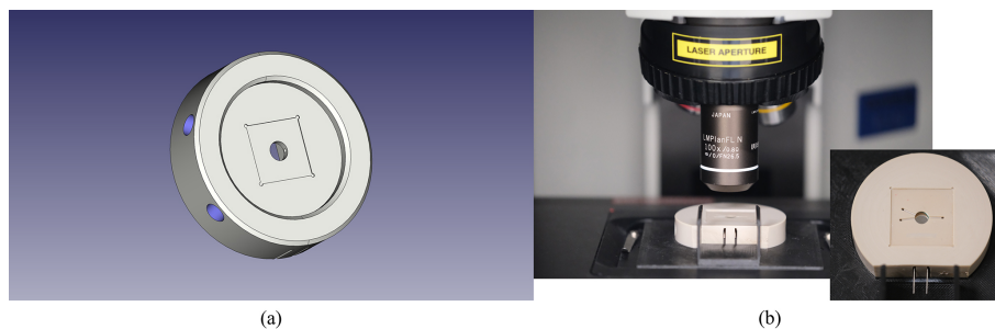
Figure 1. Details on the experimental set-up of the QCM-Raman approach. (a) 3D-Drawing of QCM-Flow-Channel in which the sensor is placed from below (figure by Holger Schürle). (b) Experimental set-up of flow cell under Raman microscope.
