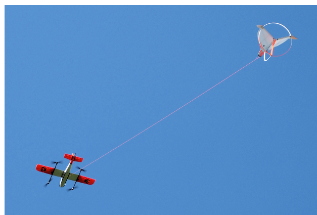
Figure 4. The 3-component Louhi EM receiver is being towed by a Coot VTOL drone in the Lintumaansuo EM test survey near Oulu, Finland, in June 2024 (Photo by Markku Pirttijärvi).
