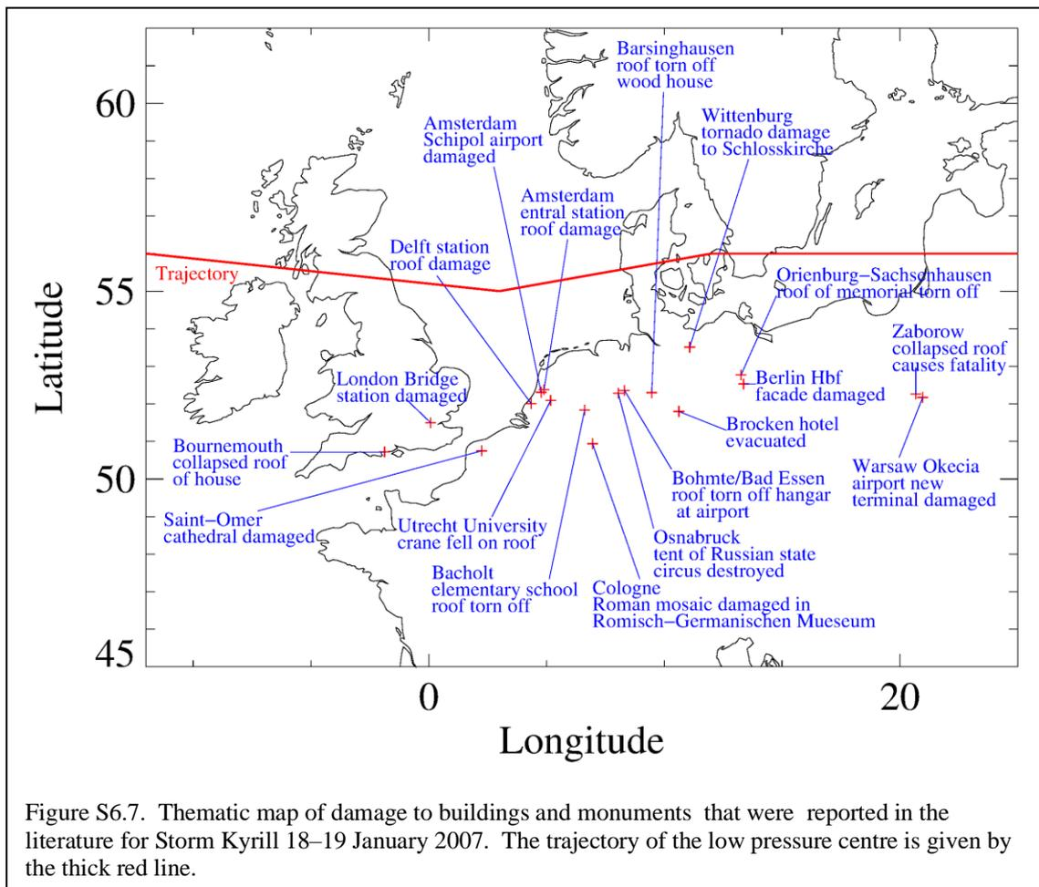
Figure S6.7. Thematic map of damage to buildings and monuments that were reported in the literature for Storm Kyrill 18–19 January 2007. The trajectory of the low pressure centre is given by the thick red line.
