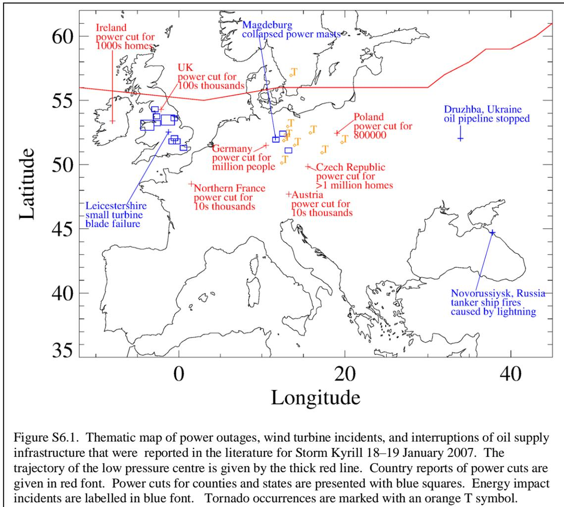
Figure S6.1. Thematic map of power outages, wind turbine incidents, and interruptions of oil supply infrastructure that were reported in the literature for Storm Kyrill 18–19 January 2007. The trajectory of the low pressure centre is given by the thick red line. Country reports of power cuts are given in red font. Power cuts for counties and states are presented with blue squares. Energy impact incidents are labelled in blue font. Tornado occurrences are marked with an orange T symbol.
