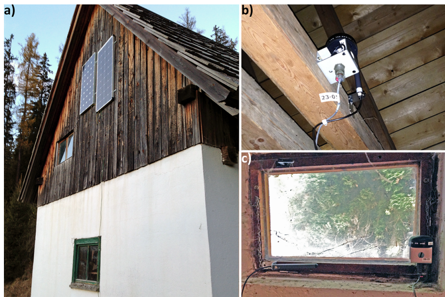
Figure 5. (a) Example of solar panel mounting (A019A). If required, two 100 W solar panels are mounted, usually vertically on walls or chimneys. (b) GPS and GSM antenna mounted indoors below wooden roof (A018A). (c) GPS and GSM antenna mounted indoors close to window (A331A).
