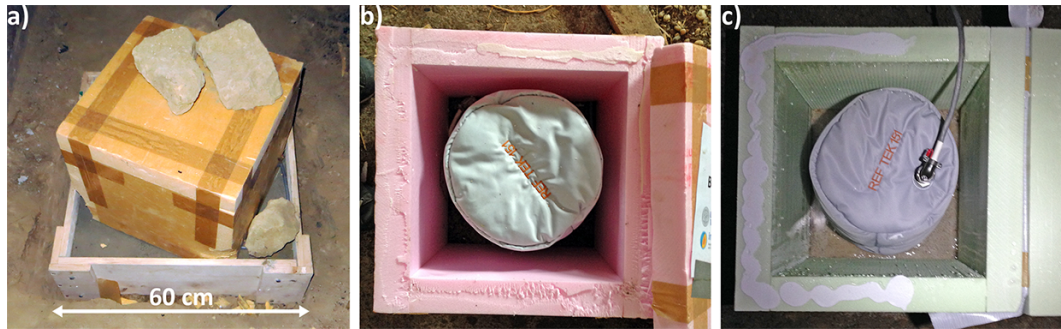
Figure 2. (a) Example of a concrete base if no solid ground is available (A006A). (b) and (c) Two-layer thermal insulation comprising a microfleece bag inside a styrofoam box. The box is glued to the ground with silicon. (b) Reftek 151 Type A sensor with connector at the bottom. (c) Reftek 151 Type B sensor with connector at the top.
